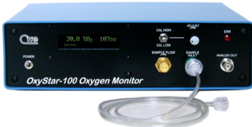
The OxyStar-100 is a fast-response, high accuracy oxygen analyzer for respiratory monitoring, hypoxic gas studies, or general laboratory use. It features a measurement range of 0 - 100% O<sub>2</sub>, with a resolution of 0.1%. Sample flow is adjustable over a 10 - 200ml/min range, making respiratory oxygen measurements possible on small as well as larger animals and human subjects.
