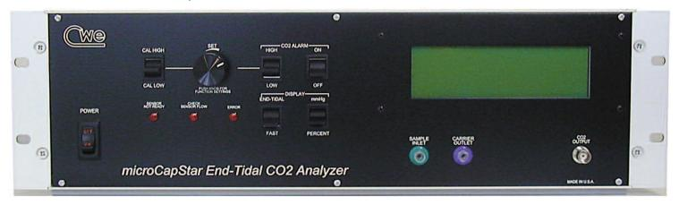
he MICROCAPSTAR End-Tidal Carbon Dioxide Analyzer provides accurate end-tidal or continuous measurement of expired CO2 in animals as small as mice. It features very low sample flow requirements, rapid response time, and long-term stability. Respiratory rate (RR) is computed using the excursions of the CO<sub>2</sub> waveform. The CO<sub>2</sub> and RR measurements, as well as a trend plot of the end-tidal values, are displayed on the graphics LCD screen.
