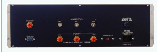
Rear-panel view of the GSM-3 Gas Mixer, showing the three gas inlet connections and the mixture outlet to the left (1/4" quick push/pull connectors). The three BNC jacks provide an analog voltage corresponding to the concentration of each input gas in the programmed mixture.
