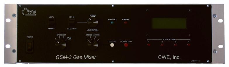
The GSM-3 Gas Mixer is a versatile and accurate device for creating custom respiratory gas mixtures. Any three gasses can be connected as inputs, and the output is the user-programmed mixture of these gasses. The instrument can operate in a stand-alone mode, with mixture programming done from the front panel controls, or it can be controlled using an attached computer running the supplied software. Besides the mixing function, the GSM-3 can operate as an accurate flow source for a single gas.
